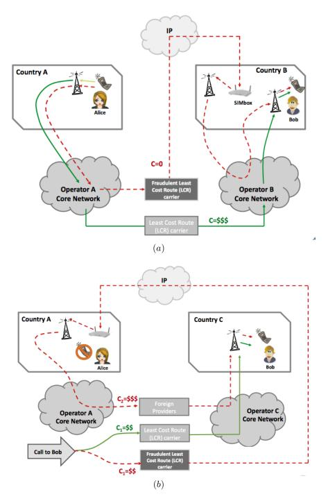
Fig. 1. Two examples of one-hope SIM-box bypass fraud: (a) hijacking of an international call (b) hijacking and re-injecting of an international call.
